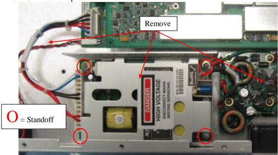
5. Install new AC power supply (PS-0000065), power harness (CA-0000564), new ground cable (PL/6140), insulator cover paper (FP/8393-1), high voltage label (LB/DNGR-HV40X28) and AC input filter (PL-0000852). See pictures below.
