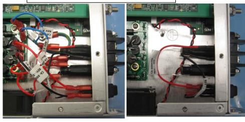
3. Remove the two (2) mounting screws and ground lug nuts. Remove the DC input and install the AC input (PF-0000001). Install two (2) fuses (FS-0000032) into the fuse housing.
